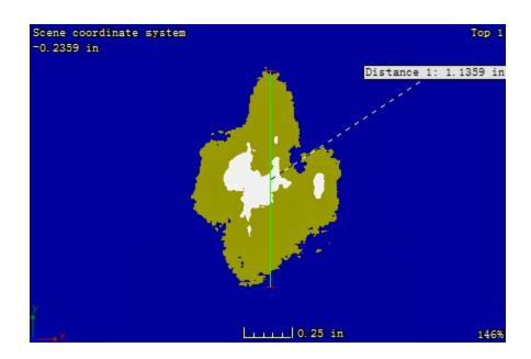
Figure C. 36: CT image at the plane with the largest damage size in sample 2-5 (located 2.47 mm away from the impacted surface)
