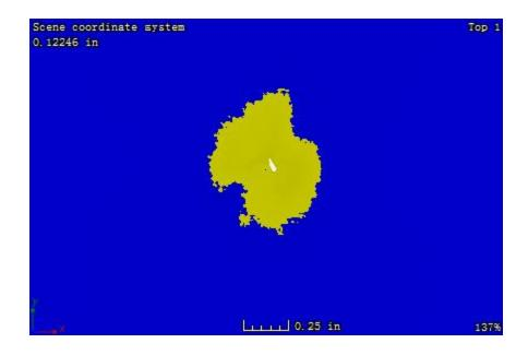
Figure B. 47: CT image at the plane located 1.37 mm away from the impacted surface of sample 1-6
