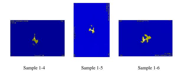
Figure 3. 40: CT image at the plane located 3.37 mm away from the impacted surface
