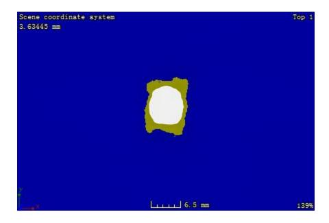
Figure C. 3: CT image at the plane located 0.47 mm away from the impacted surface of sample 2-4
