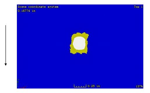
Figure B. 42: CT image at the plane located 0.22 mm away from the impacted surface of sample 1-6
