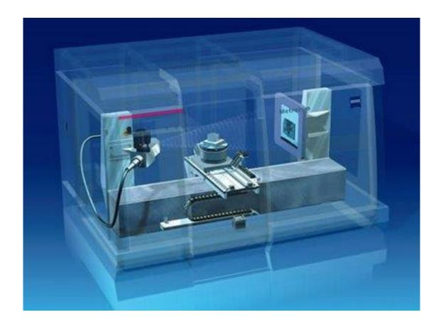
Figure 3. 4: ZEISS METROTOM 1500 System Internal Structure (Lettenbauer, 2007)
