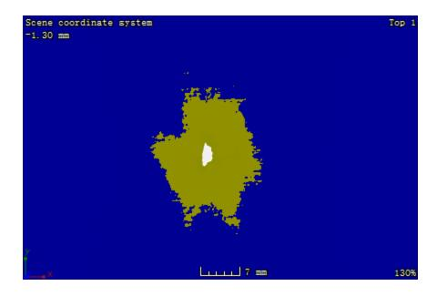
Figure B. 10: CT image at the plane located 1.62 mm away from the impacted surface of sample 1-4
