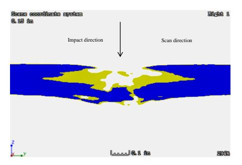
Figure B. 22: CT image in the center of sample 1-5 in the right scan direction
