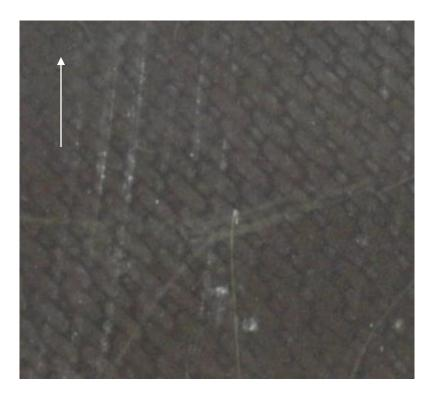
Figure 2. 7: Textile of the Specimen (the arrow indicates a 0° direction)
