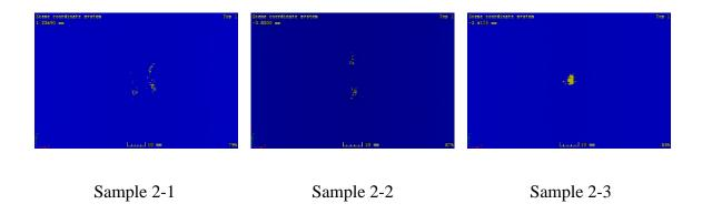
Figure 3. 20: CT image at the plane located 2.37 mm away from the impacted surface
