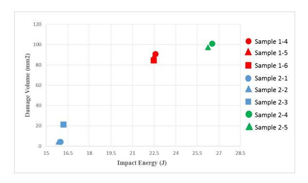
Figure 3. 64: Damage Volume vs. Impact Energy
