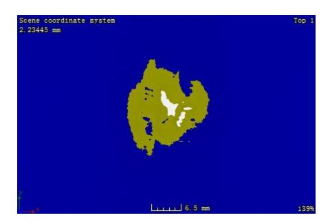
Figure C. 9: CT image at the plane located 1.87 mm away from the impacted surface of sample 2-4
