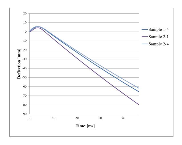
Figure 2. 25: Deflection vs. Time for Three Representative Specimens.
