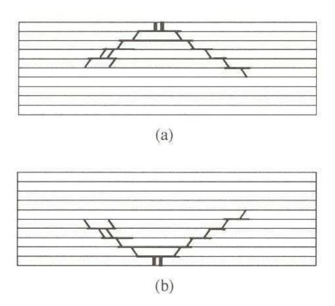
Figure 1. 16: Damage patterns of composite after impact (a) The damage pattern for thick composite (b) The damage pattern for thin composite (Abrate, 1998).
