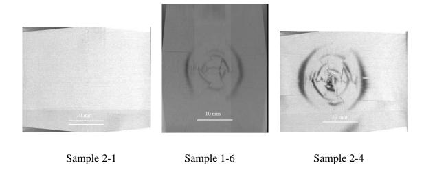
Figure 3. 76: Micro-CT image at the plane located 2.37 mm away from the impacted surface
