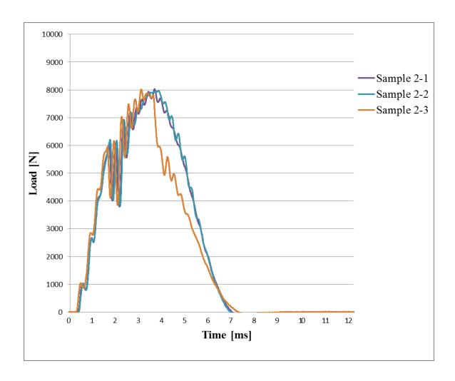
Figure 2. 14: Impact Load vs. Time for the Specimens Impacted at the Lowest Energy, 16 J.
