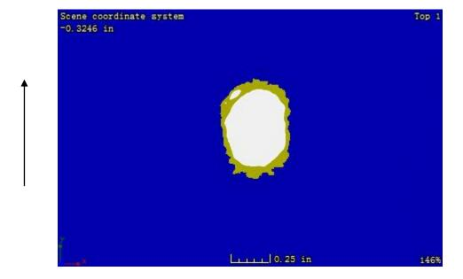
Figure C. 20: CT image at the plane located 0.22 mm away from the impacted surface of sample 2-5
