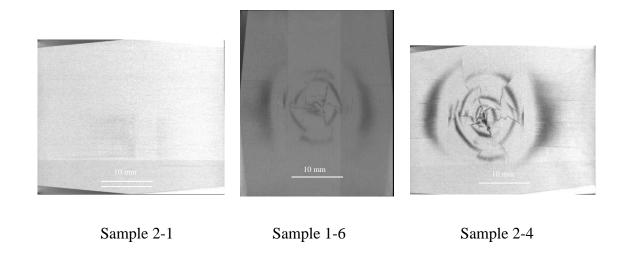
Figure 3. 75: Micro-CT image at the plane located 2.22 mm away from the impacted surface
