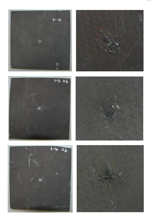
Figure 2. 27: Specimens Impacted at the Intermediate Energy, 22.5.
