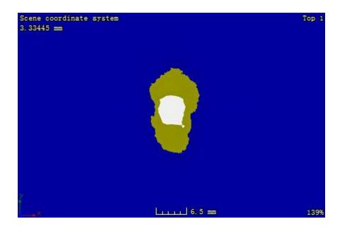
Figure C. 5: CT image at the plane located 0.77 mm away from the impacted surface of sample 2-4
