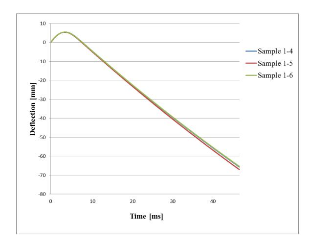
Figure 2. 19: Deflection vs. Time for the Specimens Impacted at the Intermediate Energy, 22.5 J.
