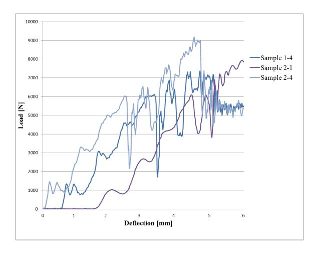
Figure 2. 24: Impact Load vs. Deflection for Three Representative Specimens.
