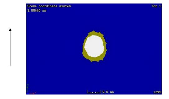
Figure C. 2: CT image at the plane located 0.22 mm away from the impacted surface of sample 2-4
