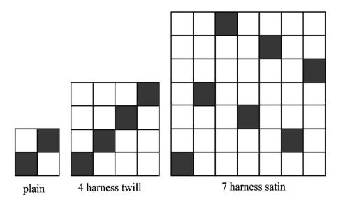
Figure 1. 1: Three fundamental ways to weave for woven fabric composites (Onal, 2007)
