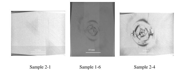
Figure 3. 73: Micro-CT image at the plane located 1.62 mm away from the impacted surface
