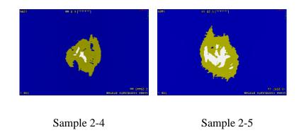
Figure 3. 53: CT image at the plane located 1.87 mm away from the impacted surface
