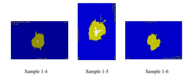
Figure 3. 32: CT image at the plane located 1.37 mm away from the impacted surface
