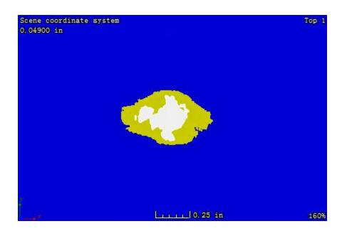
Figure B. 25: CT image at the plane located 0.47 mm away from the impacted surface of sample 1-5
