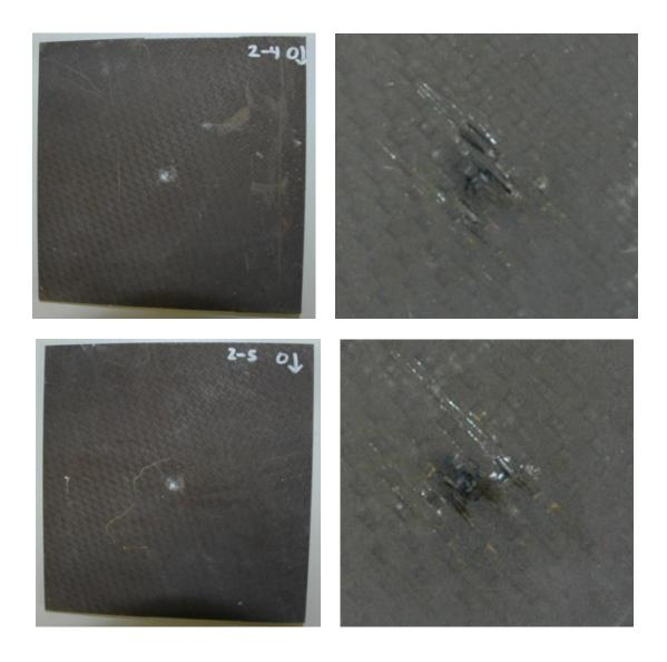
Figure 2. 28: Specimens Impacted at the Highest Energy, 26 J.
