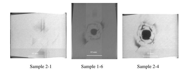
Figure 3. 69: Micro-CT image at the plane located 0.62 mm away from the impacted surface
