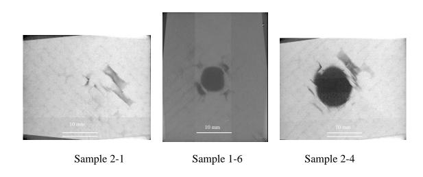
Figure 3. 67: Micro-CT image at the plane located 0.22 mm away from the impacted surface
