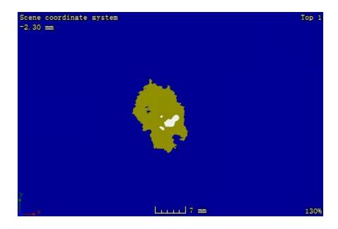
Figure B. 6: CT image at the plane located 0.62 mm away from the impacted surface of sample 1-4
