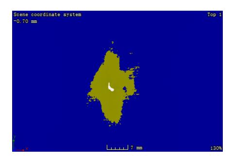
Figure B. 12: CT image at the plane located 2.22 mm away from the impacted surface of sample 1-4
