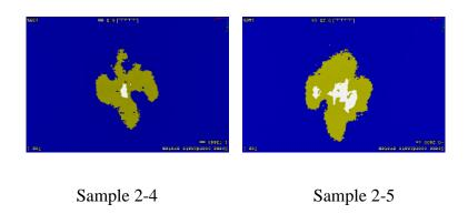
Figure 3. 55: CT image at the plane located 2.37 mm away from the impacted surface
