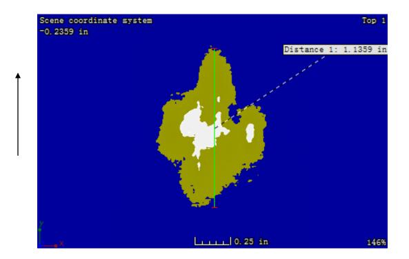
Figure 3. 63: CT image at the plane with the largest damage size in sample 2-5 (located 2.47 mm away from the impacted surface)
