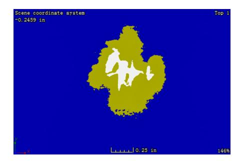
Figure C. 28: CT image at the plane located 2.22 mm away from the impacted surface of sample 2-5
