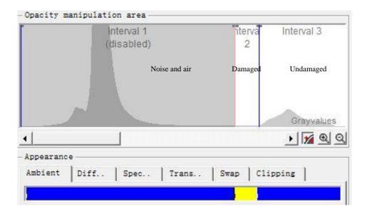
Figure 3. 10: Gray-Values Setting of samples scanned using the ZEISS METROTOM 1500.
