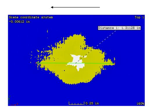
Figure 3. 44: CT image at the plane with the largest damage size in sample 1-5 (located 1.87 mm away from the impacted surface)
