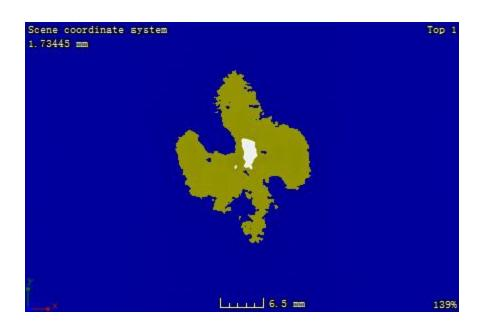
Figure C. 11: CT image at the plane located 2.37 mm away from the impacted surface of sample 2-4
