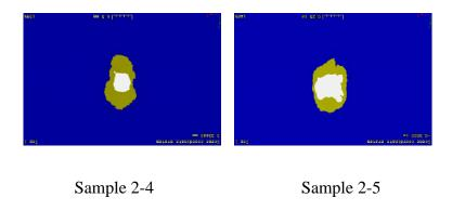
Figure 3. 49: CT image at the plane located 0.77 mm away from the impacted surface
