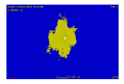
Figure B. 51: CT image at the plane located 2.37 mm away from the impacted surface of sample 1-6
