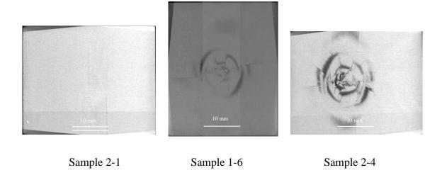
Figure 3. 72: Micro-CT image at the plane located 1.37 mm away from the impacted surface
