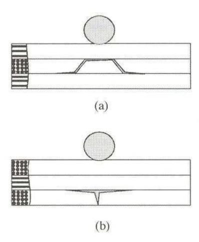
Figure 1. 15: Two types of matrix Cracks (a) Tensile crack (b) Shear crack (Abrate, 1998).
