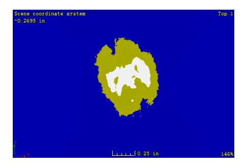
Figure C. 26: CT image at the plane located 1.62 mm away from the impacted surface of sample 2-5
