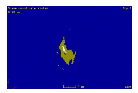
Figure B. 16: CT image at the plane located 3.12 mm away from the impacted surface of sample 1-4
