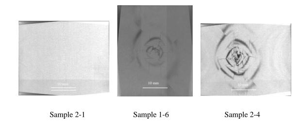
Figure 3. 79: Micro-CT image at the plane located 3.12 mm away from the impacted surface
