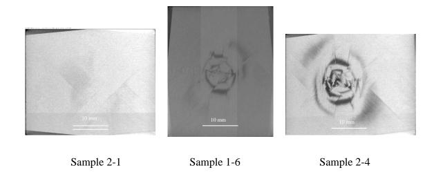
Figure 3. 71: Micro-CT image at the plane located 1.07 mm away from the impacted surface
