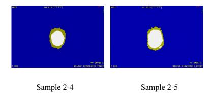
Figure 3. 46: CT image at the plane located 0.22 mm away from the impacted surface
