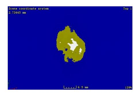
Figure C. 7: CT image at the plane located 1.37 mm away from the impacted surface of sample 2-4
