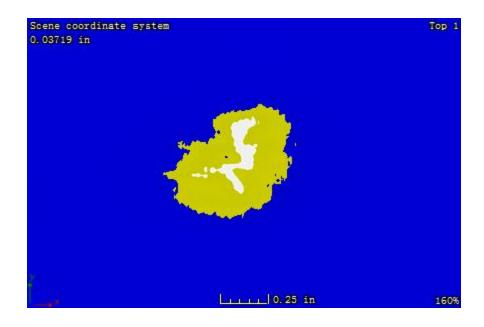
Figure B. 27: CT image at the plane located 0.77 mm away from the impacted surface of sample 1-5
