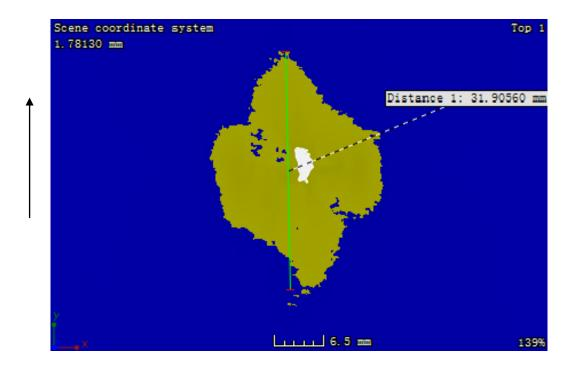
Figure 3. 62: CT image at the plane with the largest damage size in sample 2-4 (located 2.43 mm away from the impacted surface)
