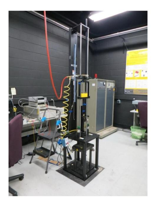
Figure 2. 1: Instron 8200 Impact Tester
