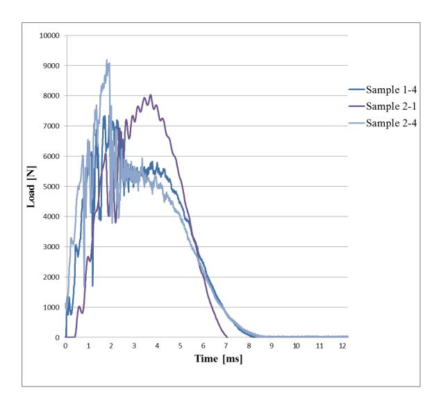
Figure 2. 23: Impact Load vs. Time for Three Representative Specimens.
