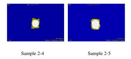
Figure 3. 47: CT image at the plane located 0.47 mm away from the impacted surface
