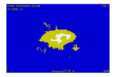
Figure B. 33: CT image at the plane located 2.37 mm away from the impacted surface of sample 1-5
