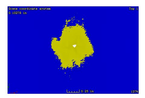
Figure B. 49: CT image at the plane located 1.87 mm away from the impacted surface of sample 1-6
