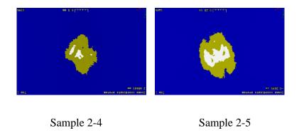
Figure 3. 52: CT image at the plane located 1.62 mm away from the impacted surface
