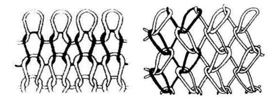
Figure 1. 5: Weft (left) and warp (right) knitted fabrics (P. Tan, 1997)
