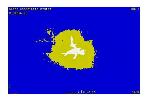
Figure B. 29: CT image at the plane located 1.37 mm away from the impacted surface of sample 1-5
