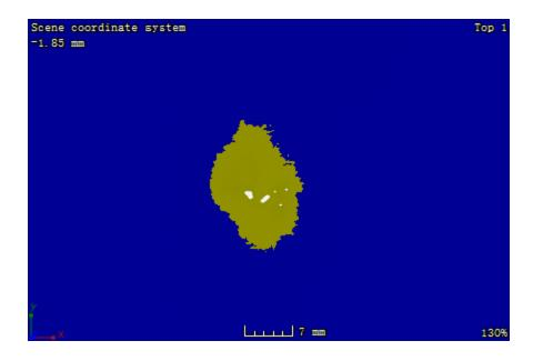
Figure B. 8: CT image at the plane located 1.07 mm away from the impacted surface of sample 1-4
