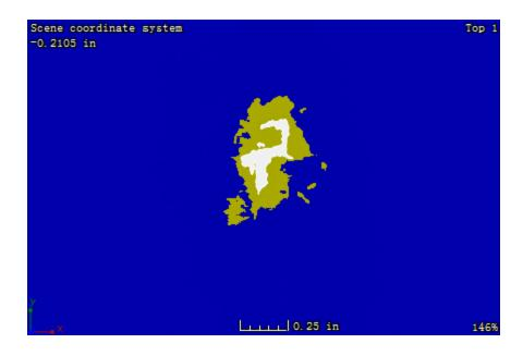
Figure C. 32: CT image at the plane located 3.12 mm away from the impacted surface of sample 2-5
