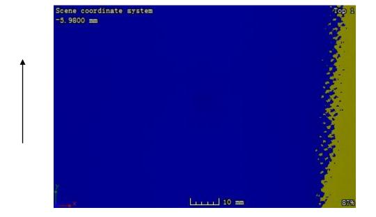
Figure A. 8: CT image at the plane located 0. 22 mm away from the impacted surface of sample 2-2
