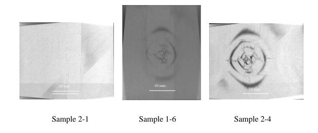
Figure 3. 77: Micro-CT image at the plane located 2.67 mm away from the impacted surface
