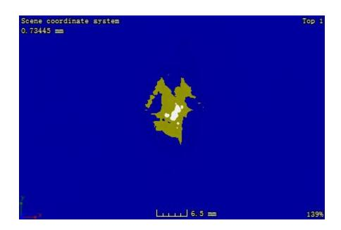
Figure C. 15: CT image at the plane located 3.37 mm away from the impacted surface of sample 2-4
