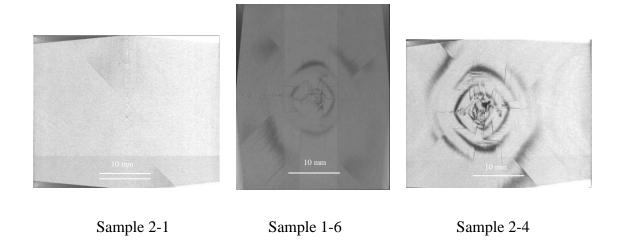
Figure 3. 78: Micro-CT image at the plane located 2.92 mm away from the impacted surface
