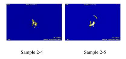
Figure 3. 61: CT image at the plane located 3.87 mm away from the impacted surface
