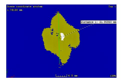
Figure C. 18: CT image at the plane with the largest damage size in sample 2-4 (located 2.43 mm away from the impacted surface)
