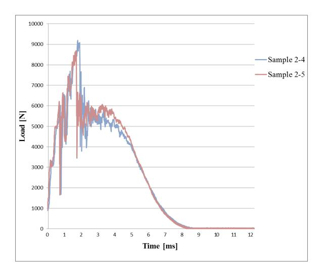
Figure 2. 20: Impact Load vs. Time for the Specimens Impacted at the Highest Energy,  $26\,\mathrm{J}.$
