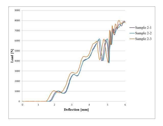
Figure 2. 15: Impact Load vs. Deflection for the Specimens Impacted at the Lowest Energy, 16 J.
