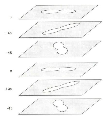
Figure 1. 14: Orientation of delaminations (Abrate, 1998).
