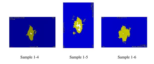
Figure 3. 36: CT image at the plane located 2.37 mm away from the impacted surface
