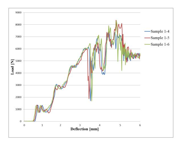
Figure 2. 18: Impact Load vs. Deflection for the Specimens Impacted at the Intermediate Energy, 22.5 J.
