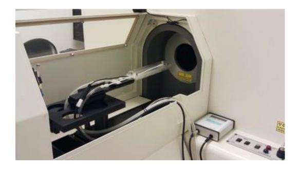
Figure 3. 7: The Scanner Bed in the Siemens MicroCAT II Scanner (MicroCAT II, 2014)
