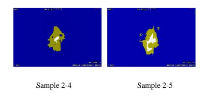
Figure 3. 57: CT image at the plane located 2.92 mm away from the impacted surface
