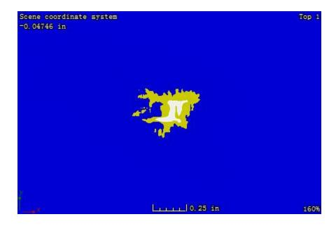
Figure B. 35: CT image at the plane located 2.92 mm away from the impacted surface of sample 1-5
