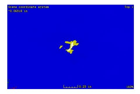
Figure B. 37: CT image at the plane located 3.37 mm away from the impacted surface of sample 1-5
