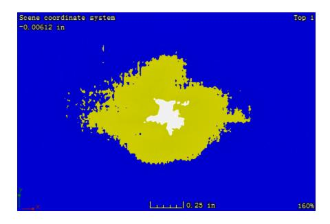
Figure B. 31: CT image at the plane located 1.87 mm away from the impacted surface of sample 1-5
