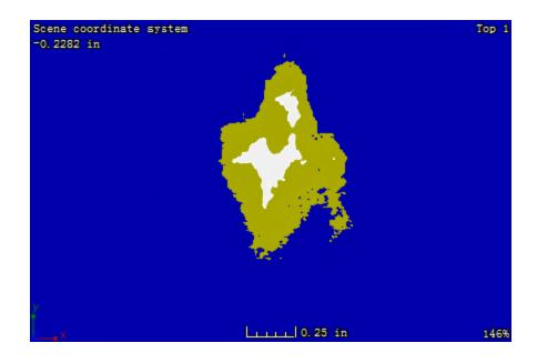
Figure C. 30: CT image at the plane located 2.67 mm away from the impacted surface of sample 2-5
