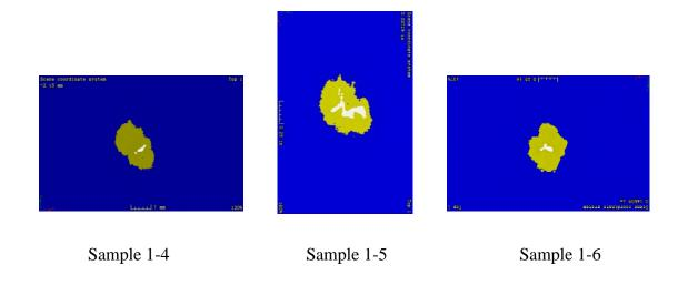
Figure 3. 30: CT image at the plane located 0.77 mm away from the impacted surface
