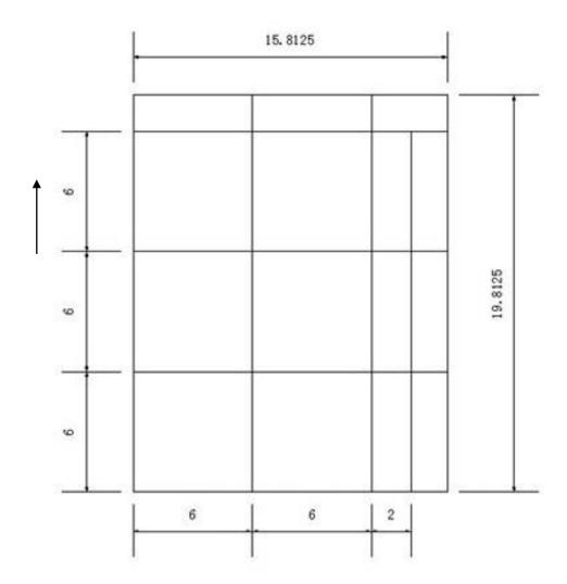
Figure 2. 8: Cutting Layout of Composite Panel 1 (the Arrow Indicates 0° Direction)
