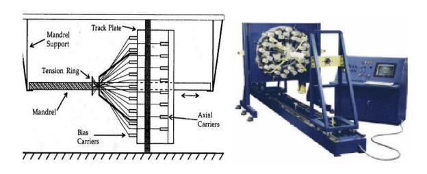
Figure 1. 9: The cylindrical mandrel to manufacture a braided composite (Chretien, 2002)
