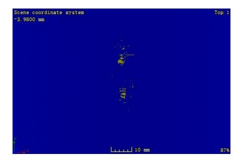
Figure A. 10: CT image at the plane located 2.22 mm away from the impacted surface of sample 2-2
