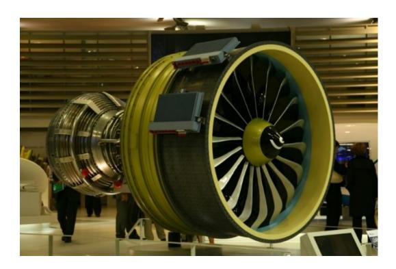
Figure 1. 12: CFM International new LEAP engine with 18 blades made from 3D woven composite (Composites Manufacturing Online, 2013)
