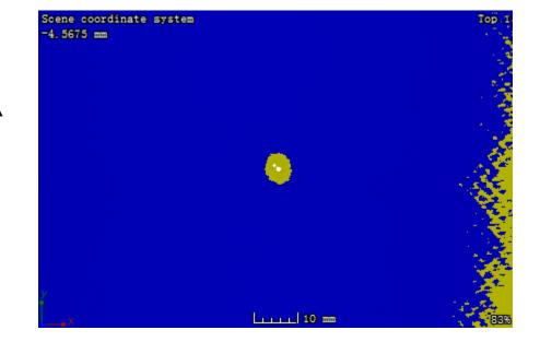
Figure A. 15: CT image at the plane located 0. 22 mm away from the impacted surface of sample 2-3
