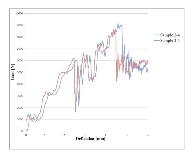
Figure 2. 21: Impact Load vs. Deflection for the Specimens Impacted at the Highest Energy, 26 J.
