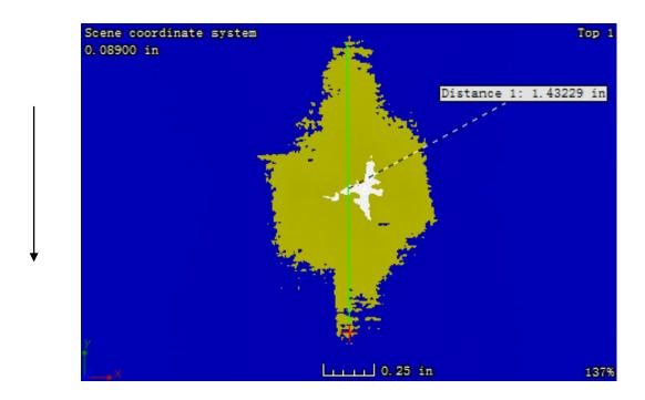
Figure 3. 45: CT image at the plane with the largest damage size in sample 1-6 (located 2.22 mm away from the impacted surface)
