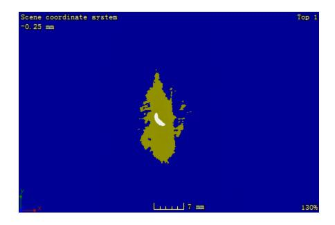
Figure B. 14: CT image at the plane located 2.67 mm away from the impacted surface of sample 1-4
