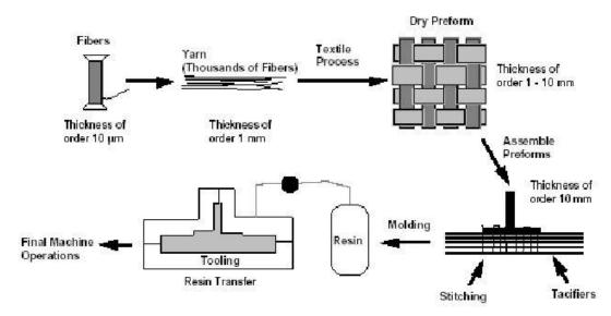
Figure 1. 8: Procedure to manufacture the textile composite (Chretien, 2002)
