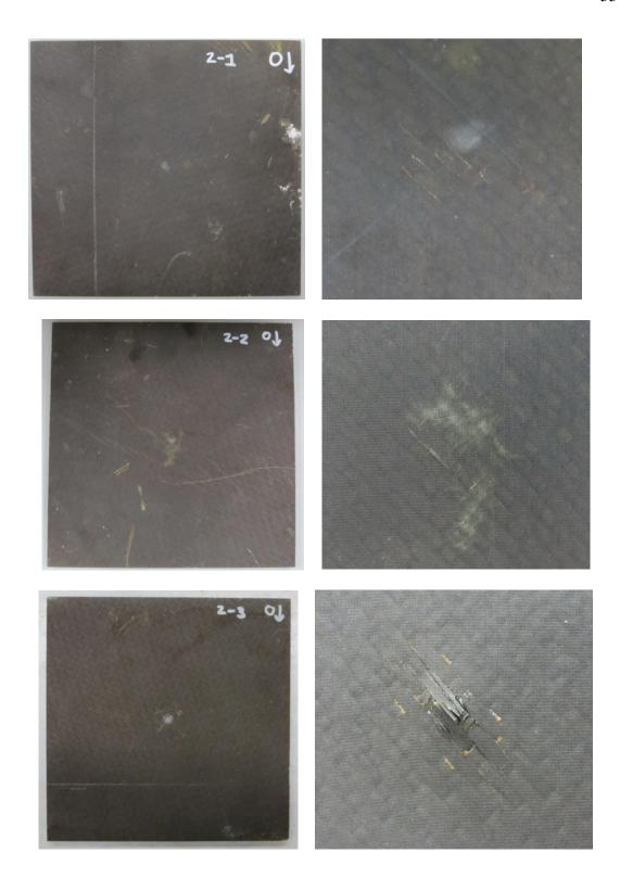
Figure 2. 26: Specimens Impacted at the Lowest Energy, 16 J.
