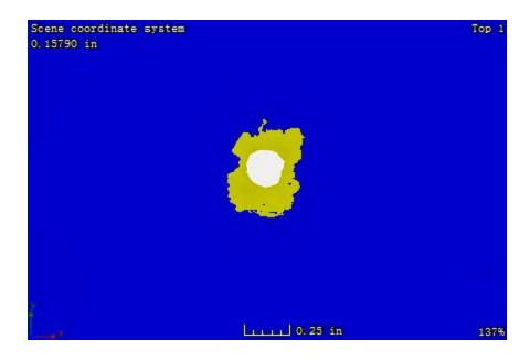
Figure B. 43: CT image at the plane located 0.47 mm away from the impacted surface of sample 1-6
