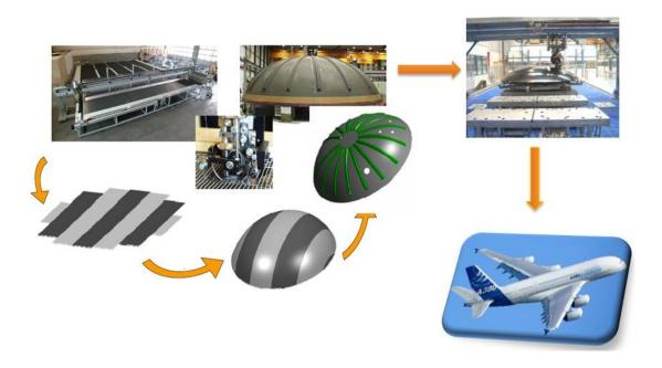
Figure 1. 11: Procedure to manufacture the textile composite pressure bulkhead (Wordpress, 2013)
