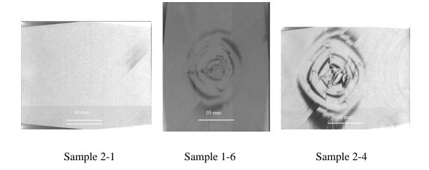
Figure 3. 82: Micro-CT image at the plane located 3.87 mm away from the impacted surface
