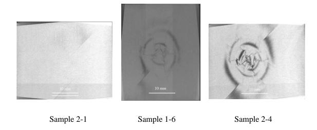
Figure 3. 74: Micro-CT image at the plane located 1.87 mm away from the impacted surface
