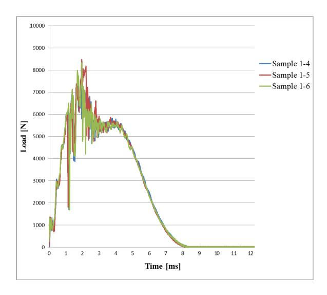
Figure 2. 17: Impact Load vs. Time for the Specimens Impacted at the Intermediate Energy, 22.5 J.
