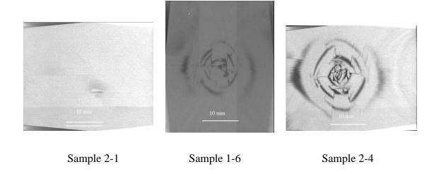
Figure 3. 80: Micro-CT image at the plane located 3.37 mm away from the impacted surface
