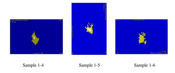
Figure 3. 38: CT image at the plane located 2.92 mm away from the impacted surface
