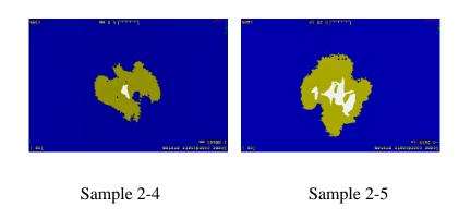
Figure 3. 54: CT image at the plane located 2.22 mm away from the impacted surface
