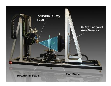
Figure 3. 1: General Operation and Major Components of the Modern Industrial CT System (Makeev 2011)
