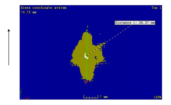
Figure 3. 43: CT image at the plane with the largest damage size in sample 1-4 (located 2.17 mm away from the impacted surface)
