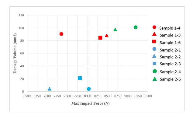
Figure 3. 65: Damage Volume vs. Max Impact Force
