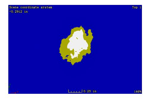
Figure C. 24: CT image at the plane located 1.07 mm away from the impacted surface of sample 2-5
