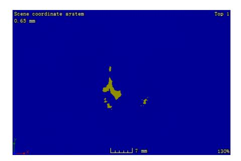
Figure B. 18: CT image at the plane located 3.57 mm away from the impacted surface of sample 1-4
