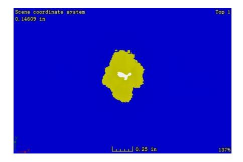
Figure B. 45: CT image at the plane located 0.77 mm away from the impacted surface of sample 1-6
