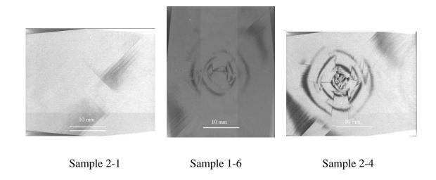
Figure 3. 81: Micro-CT image at the plane located 3.57 mm away from the impacted surface
