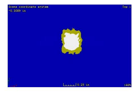
Figure C. 22: CT image at the plane located 0.62 mm away from the impacted surface of sample 2-5
