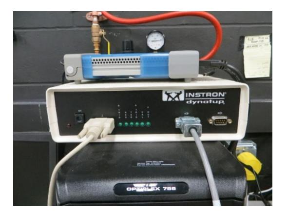
Figure 2. 6: Impact Tester Signal Conditioning Box
