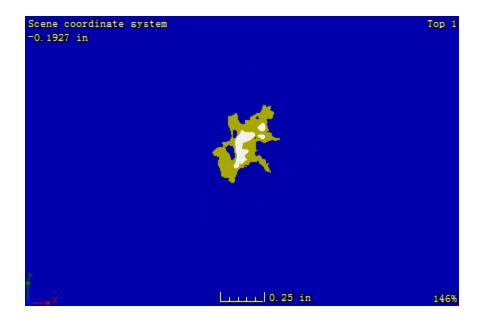
Figure C. 34: CT image at the plane located 3.57 mm away from the impacted surface of sample 2-5
