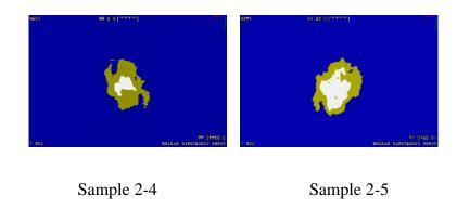
Figure 3. 50: CT image at the plane located 1.07 mm away from the impacted surface
