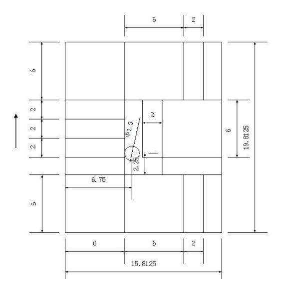
Figure 2. 9: Cutting Layout of Composite Panel 2 (the Arrow Indicates 0° Direction)
