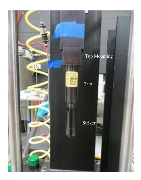
Figure 2. 5: Instrumented Load Cell
