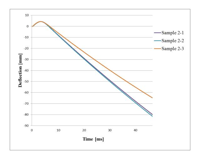
Figure 2. 16: Deflection vs. Time for the Specimens Impacted at the Lowest Energy, 16 J.
