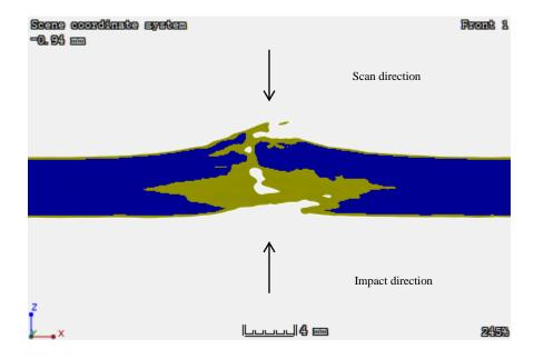
Figure B. 3: CT image in the center of sample 1-4 in the front scan direction
