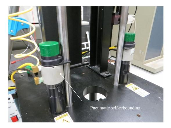
Figure 2. 2: Two Pneumatic Self-Rebounding Stoppers
