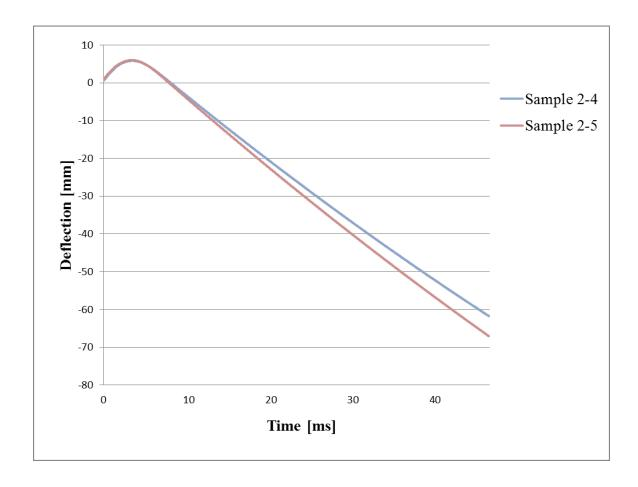
Figure 2. 22: Deflection vs. Time for the Specimens Impacted at the Highest Energy, 26 J.
