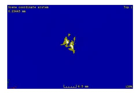
Figure C. 17: CT image at the plane located 3.87 mm away from the impacted surface of sample 2-4
